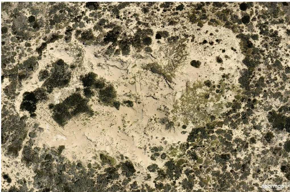
AFTER: Laying of brush material and woven geotextile cloth to provide stability and trap moving sands (B Simon)
