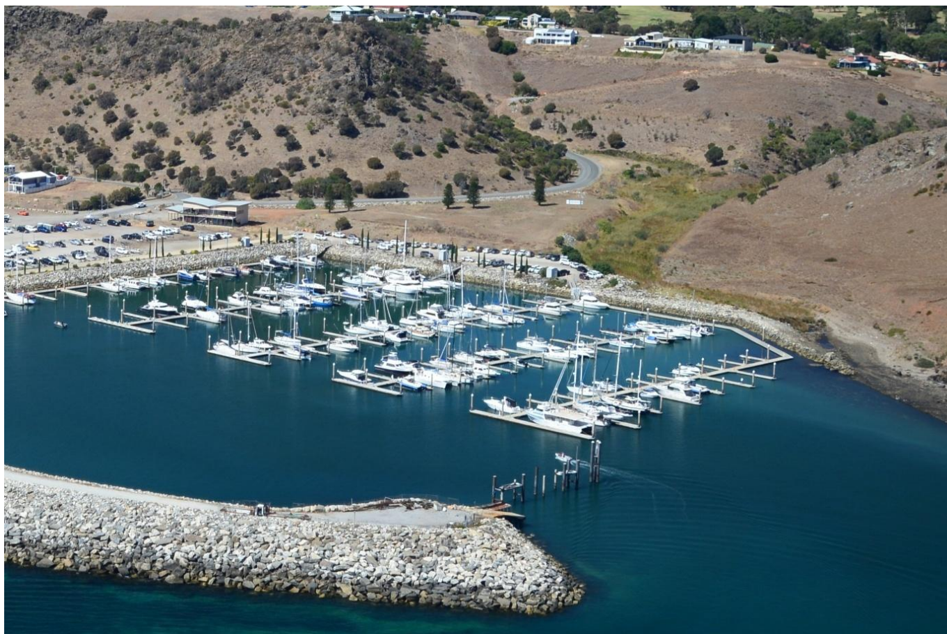
Congeratinga – Anacotilla River estuary has an altered mouth due to the construction of the Wirinna ‘Sunset Cove’ marina and has been redirected west from its natural alignment (Coast Protection Board, March 2024)
